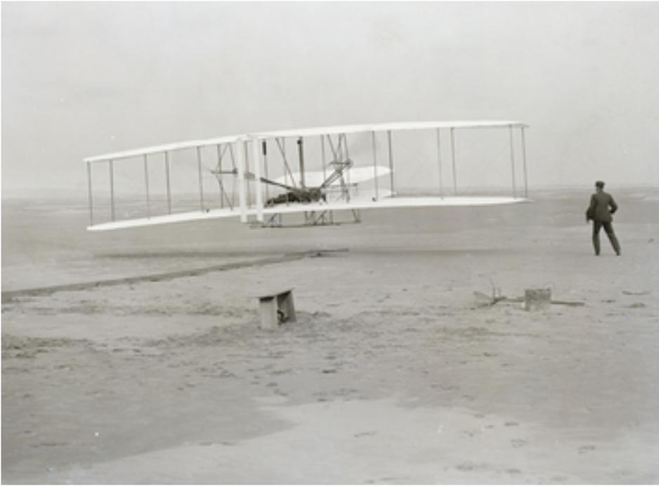
Lying flat on the lower wing of the 1903 Wright flyer, Orville Wright begins the first successful airplane flight in history as his brother Wilbur runs alongside during takeoff. The Wright brothers designed and built the flyer out of wood and cloth. It was powered by a gasoline engine of the Wrights' own design.
